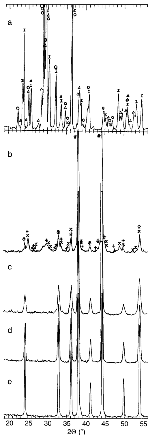
FIG. 2. XRD patterns of Sample 4 (V/Ag = 2.16) at different stages of TPR with \text{H}_2/\text{N}_2 : (a) before reduction; (b) first TPR peak; (c) second TPR peak; (d) third TPR peak; (e) after shoulder peak of TPR. In patterns, the symbols used for the phases and the numbers of JCPDS cards are as follows: I— \text{Ag}_2\text{V}_4\text{O}_{11} , 20-1385; O— \text{Ag}_2\text{V}_4\text{O}_{11-y} , 20-1386; \Delta — \text{Ag}_{1.20}\text{V}_3\text{O}_8 , 23-647; \# —Ag, 4-0783; +— \text{VO}_2 , 31-1439; \phi — \text{V}_2\text{O}_3 , 34-187; X— \text{V}_6\text{O}_{13} , 27-1318.
